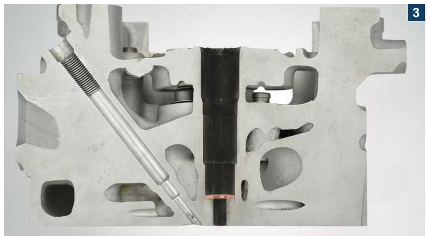
*Cylinder head cross section with soiled injector shaft*
