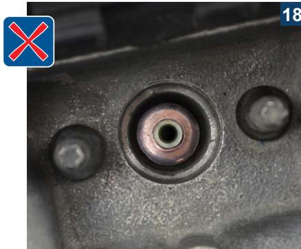
If the copper seal is already removed with the injector from the shaft, then continue with **step 2.4**.
