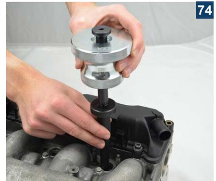
Tap gently with the slide hammer the extractor claw of the sealing ring extractor into the bore of the sealing ring.
