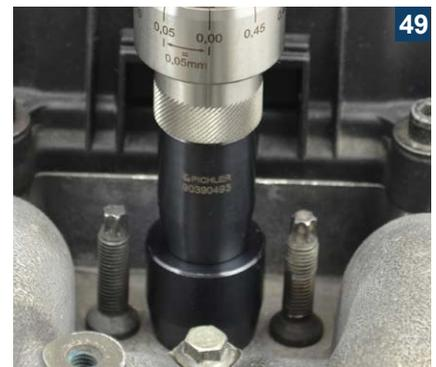
Retain the upper scale ring and turn the lower ring on the depth stop so long in a **clockwise direction**, until the stop. **50**
