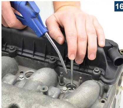
Remove the loosened deposits with a vacuum cleaner or compressed air.
