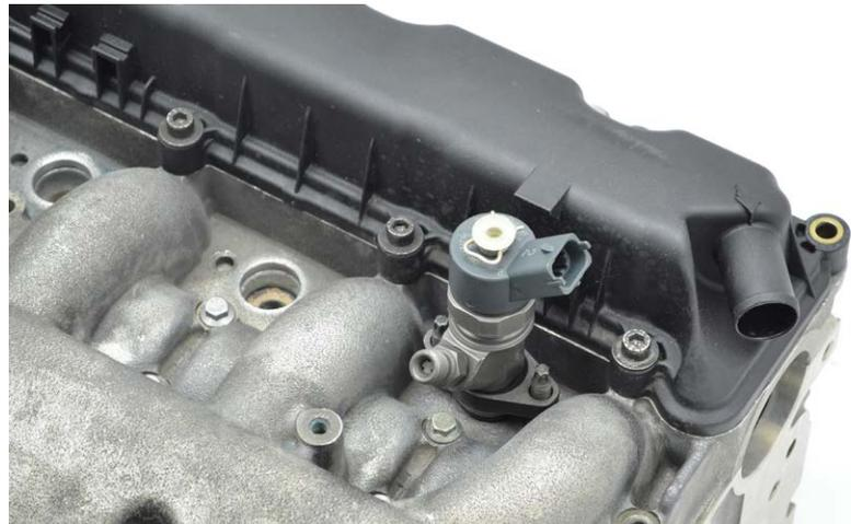
Remove the injector from the cylinder head with a suitable tool.
