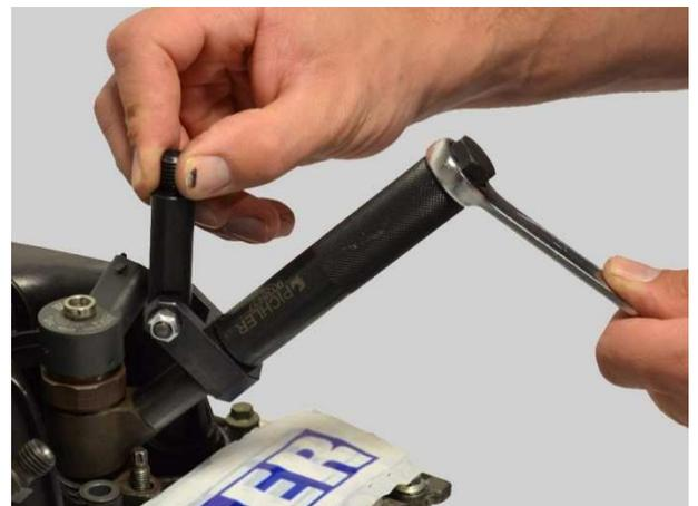
2.4 Screw the slide hammer 1030210 on the Swivel Joint 9038440.
