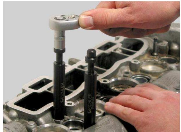
Slide the Injector sleeve 6038527 on the Seal and Injector Sleeve Drift 60385436 and slide the Centralising Ring 60385439 over the Injector sleeve.
