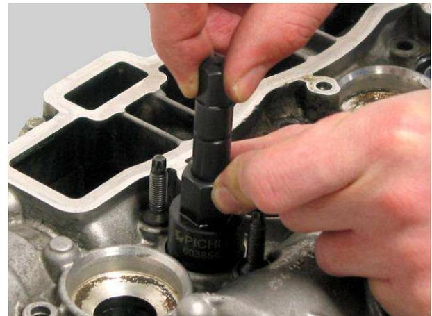
While applying a slight downward pressure turn the Cleaning Cutter with a socket 12 and ratchet until the groove on the spindle of the Cleaning Cutter has completely disappeared in the Guide.
