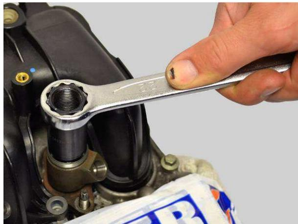
Screw the Sleeve Adaptor 60384417 on the thread for the solenoid valve and tighten it with suitable spanner 32.
