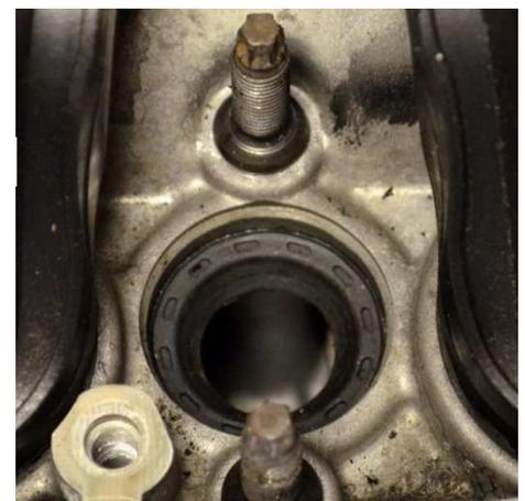
If the injector could be removed without the injector sleeve being pulled from the cylinder head (**picture A**), only the steps marked with
