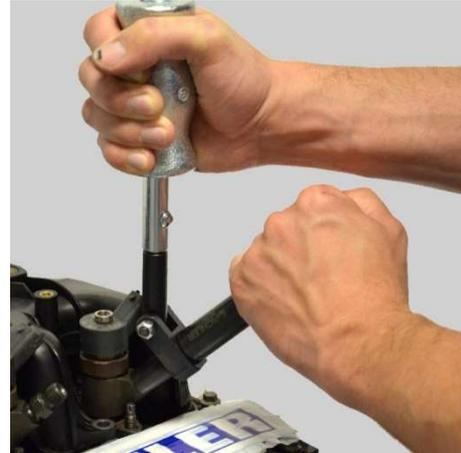
2.5 Remove the injector by jolting the Loosening Lever and simultaneously hitting with the slide hammer.
