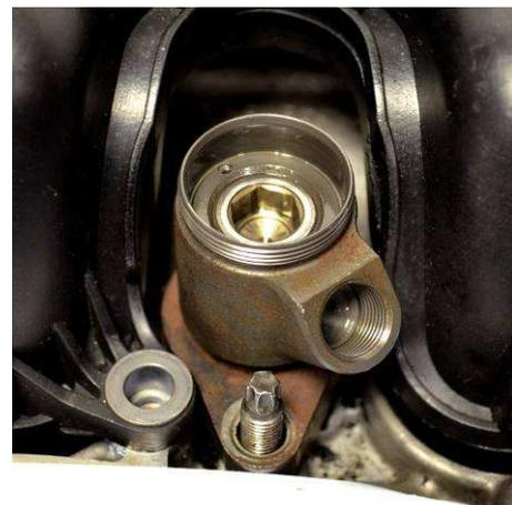
Unscrew and remove with the Pilot Valve Socket 60384172 and a ratchet  $\frac{1}{4}$ " the hexagon screw.
