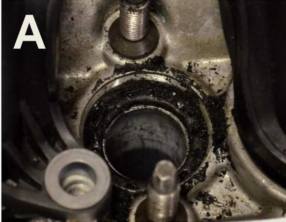
In some cases it may happen that the injector sleeve is pulled from the cylinder head with the injector (**picture B**). If so, all steps have to be carried out in the correct sequence.
