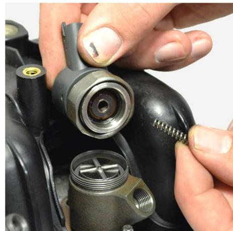
Remove the loose small parts with a magnet, so that only the hexagon screw is visible.
