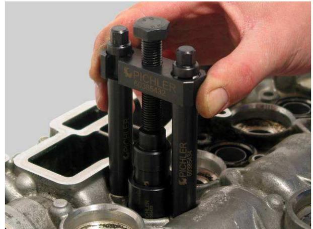
By turning the spindle with a 19mm socket and a ratchet and at the same time holding the bridge with a spanner 20, press the injector sleeve 60385427 in the cylinder head.
