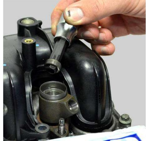
Push the injector needle extractor 6038472E in the injector. Tighten the hex nut with a spanner 14 and extract the injector needle.
