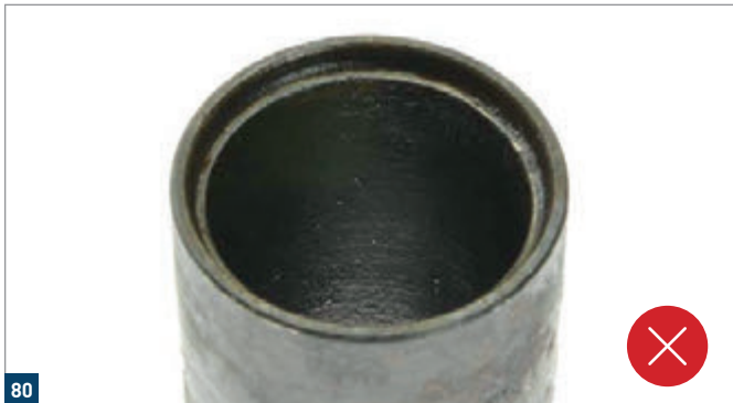
Retainer ring is not in the sleeve
