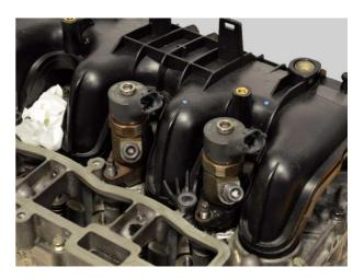
1.2 Seal all openings with tape or similar and remove with a slotted screwdriver and a vacuum cleaner, the dirt and carbon deposits around the injector.
