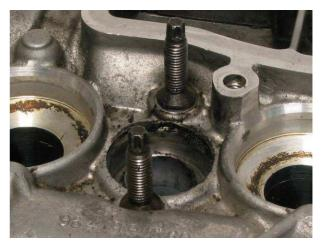
Place the Cleaning Cutter and Guide *60385422* in the sealing ring seat and by rotating it with ratchet with socket 19 remove the oil and carbon deposits from the seat.
