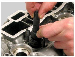
While applying a slight downward pressure turn the Cleaning Cutter with a socket 12 and ratchet until the groove on the spindle of the Cleaning Cutter has completely disappeared in the Guide.
