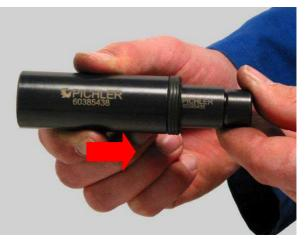
Slide the assembly in the injector sleeve, screw up the spindle of the Support Bridge 60385432 and place the Bridge on the Legs 60385434.
