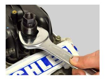
Screw the Box Nut Adaptor 60384413 on the Sleeve Adaptor and tighten it with suitable spanner 32.
