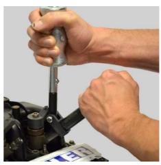
2.5 Remove the injector by jolting the Loosening Lever and simultaneously hitting with the slide hammer.
