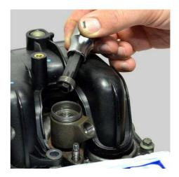
Push the injector needle extractor 6038472E in the injector. Tighten the hex nut with a spanner 14 and extract the injector needle.
