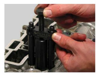
By turning the Spindle with a socket 19 and a ratchet press the sealing ring completely in the cylinder head.
