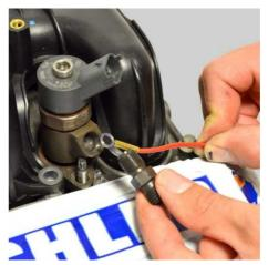
2.3 Screw the Loosening Lever 9038437 with Swivel Joint 9038440 in the bore of the diesel connector.
