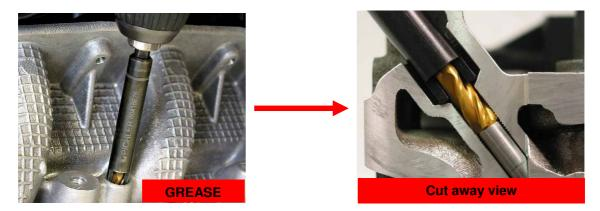
Free the sleeve of metal swarf with a magnet or compressed air.
