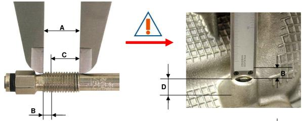
No protrusion: A - D =yet to be drilled depth protrusion: C - D =yet to be drilled depth
