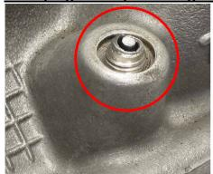
Glow plug with no protruding thread
