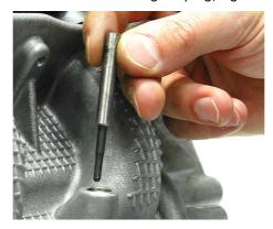
Insert the Special Reamer Ø9 (p/n 60421010) into the glow plug shaft.
