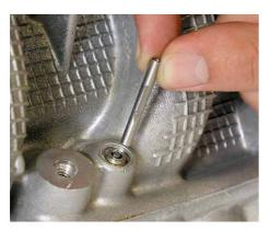
D) Hammer the Drill Sleeve (p/n 6041641) only half way in.
