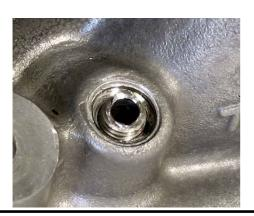
**K)** While withdrawing the drill repeatedly, drill till the stop on the cylinder head or till a clear resistance is perceptible.
