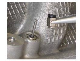
Hammer the **Stud Puller Ø2.5mm (p/n 1131025)** on the central electrode and break it off by turning it several times clockwise
