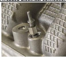
A) Place the Stud Puller Ø4.0mm (p/n: 1131040) for smooth connectors on to the central electrode and with a 1/4" ratchet break off the central electrode by turning it several times clockwise.
