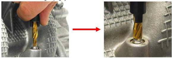
Clamp the **Drill Ø4.5mm (p/n 6041635)** with the **Tool Holder (p/n 60416675)** in a electric drill and drill about 4-5mm into the glow plug thread.
