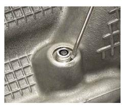
**A)** Remove the possible burr between glow plug and the central electrode.
