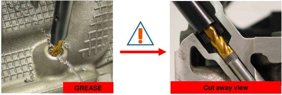
With a magnet or compressed air free the glow plug shaft of metal swarf.
