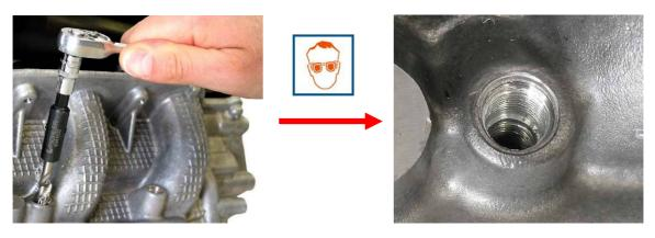
With a magnet or compressed air free the sleeve of swarf.
