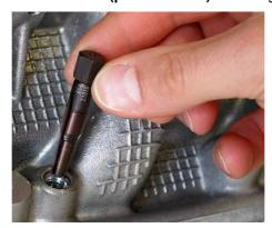
Drill with the **Special Reamer Ø9 (p/n 60421010)** and a appropriate tool deep enough (approximately 14mm) into the glow plug shaft and remove the swarf.
