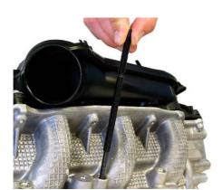
Place the Support Sleeve (p/n 60416533) over the Extraction Spindle (p/n 60416473).
