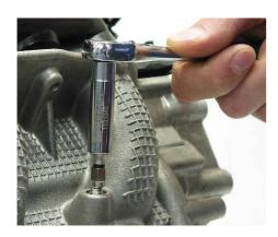
A) Place the Stud Puller Ø3.5mm (p/n 1131035) for threaded connectors on to the pin of the cap of the glow plug and hammer it on.
