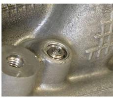
C) Hammer the Drill Sleeve (p/n 6041641) only half way in.
