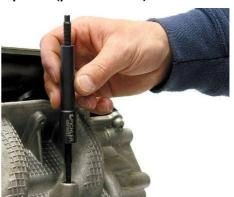
Screw the Extraction Nut (p/n 60416536) onto the Extraction Spindle (p/n 60416473) and start the extraction procedure.
