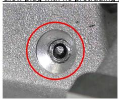
**A)** Clean the **protruding thread** of the glow plug.
