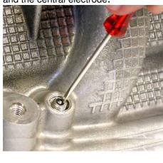
**B)** Put the **Drill Sleeve (p/n 6041641)** on the central electrode.
