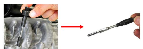
Clear the glow plug shaft of soot and debris.
