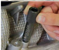
G) Clamp the Tool Holder (p/n 60416675), with clamped in Drill (p/n 6041635), in a power drill and grease it.
