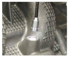
Insert the Glow Plug Reamer (p/n 6041625) into the glow plug shaft and rub the sealing seat.
