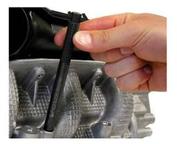
Remove the **Insert Setting Tool (p/n 6042106)** and install the new glow plug with torque as indicated by manufacturer specification.
