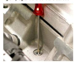
**B)** Remove the possible burr between glow plug and the central electrode.
