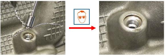
Clamp the **Tap UNF No.12x28** (p/n 6041643) into the **Adapter** (p/n 6041632) or in the tool holder **Keeper** (p/n 6041738) and cut with feeling, as deeply as possible, a thread in the glow plug.
