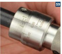
If necessary, release the lower ring, and add 0.05 mm. Repeat steps 54 to 59 as long as necessary until all deposits are removed
