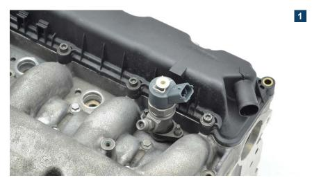
Remove the injector from the cylinder head with a suitable tool.
