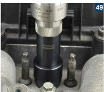
Retain the upper scale ring and turn the lower ring on the depth stop so long in a **clockwise direction**, until the stop. 50
