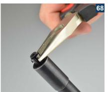
After being used several times it can happen that the four claw elements get overstretched and do not fit in the sealing ring anymore. This can be corrected by squeezing them together with a pair of long-nosed pliers.
