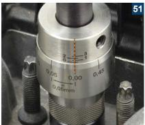
Push the injector seat milling cutter all the way in, press the depth stop on the centring cone and at the same time clamp the upper scale ring.
