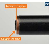
The claw is optimally adjusted when the collar protrudes minimally over the sealing ring.
