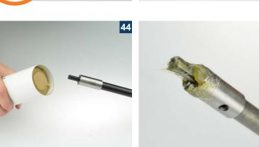
Slide it flush on to the basic device and make sure, that it's clamped on the flat spot of the basic device.
