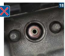
If the copper seal is already removed with the injector from the shaft, then continue with **step 2.4.**
