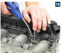
Remove the loosened deposits with a vacuum cleaner or compressed air.
