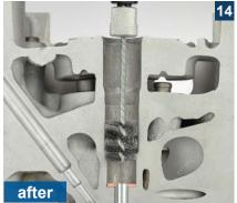
Clean the surface of the injector shaft at medium speed.
