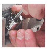
Put the reamer actuator with the interior square onto the reamer and without generating too much pressure and using a clockwork rotation clean the shaft of soot and deposits.
