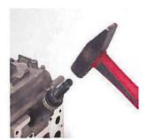
In case it is not possible to place the **Drill Sleeve** 6041745 on the cylinder head, the glow plug can be extracted with the **Adapter** 6041798 and the **Extraction Insert UNF** 1/4° 6041746 and a slide hammer.
