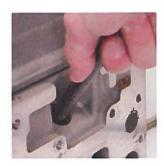
Tighten the Thread Insert with the Insert Setting Tool and remove the Insert Setting Tool.
