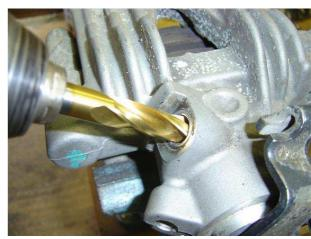
6. Depending on the repair bleeder valve used from 9353005, use the matching tap NPT 1/4" 9353014 or NPT 1/8" 9353018 and cut a thread into the caliper.
