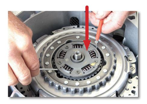
Shock with tool and soft hammer in order to ease up the snap ring for clutch pack.
