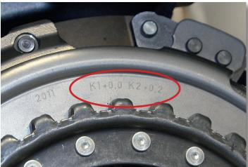
Put aside a small (K2) shim 2,40 mm Take out the tool and K2 thrust bearing
