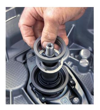
Place the new dual clutch pack carefully in place. It has to be fit into the larger splines (on the outer input shaft).
