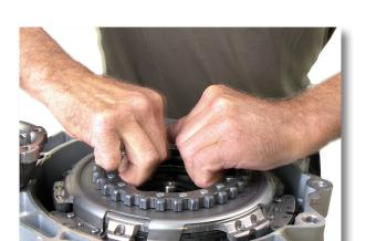
Check that the dual clutch pack is correctly in place by checking the distance between the upper edge of the outer (hollow) input shaft and the upper bearing edge. The distance must be less than 8 mm (normally approximately 7 mm).
