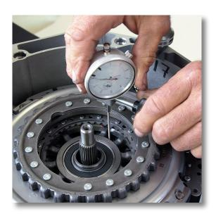
Measure the clearance of K2 by lifting the clutch plate with 2 hooks. The clearance must be 0.3 - 1.0 mm. If less, the dual clutch needs to be changed\* and reinstalled.
