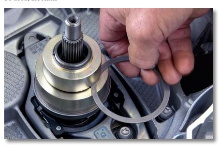
Put aside a K1 shim of proper thickness. Take out the tool
